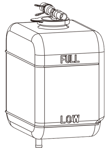
Add coolant directly to the Coolant Overflow Tank
