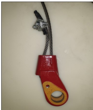
(Fig. 6) Notice the embossed arrow on the side of the becket; the wire rope goes through the narrow end following the arrow.
