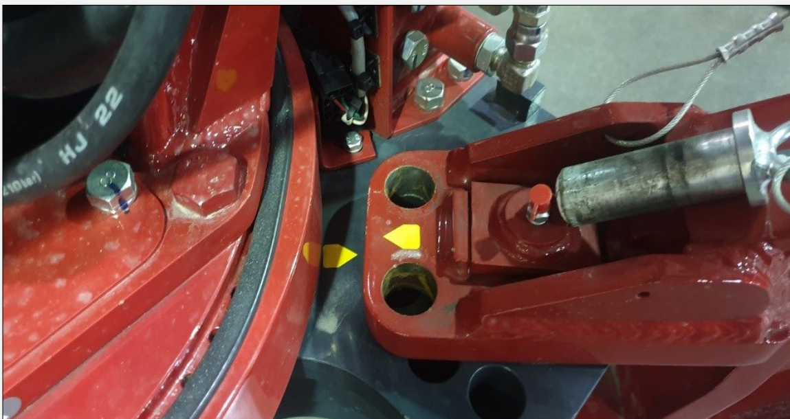
(Fig. 2): The Optimum Deployment Angle Indicator for the 095-/200-Series.
