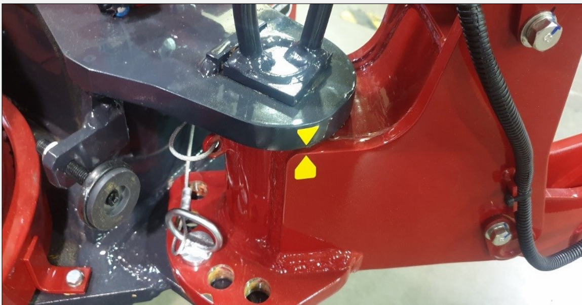
(Fig. 1): The Optimum Deployment Angle Indicator for the URW094.
