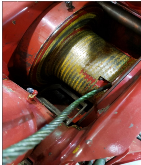
(Fig. 4): Make sure that the end is visible in the socket cutout BUT NOT protruding out of the cutout (and tangling into the stored wire rope.
