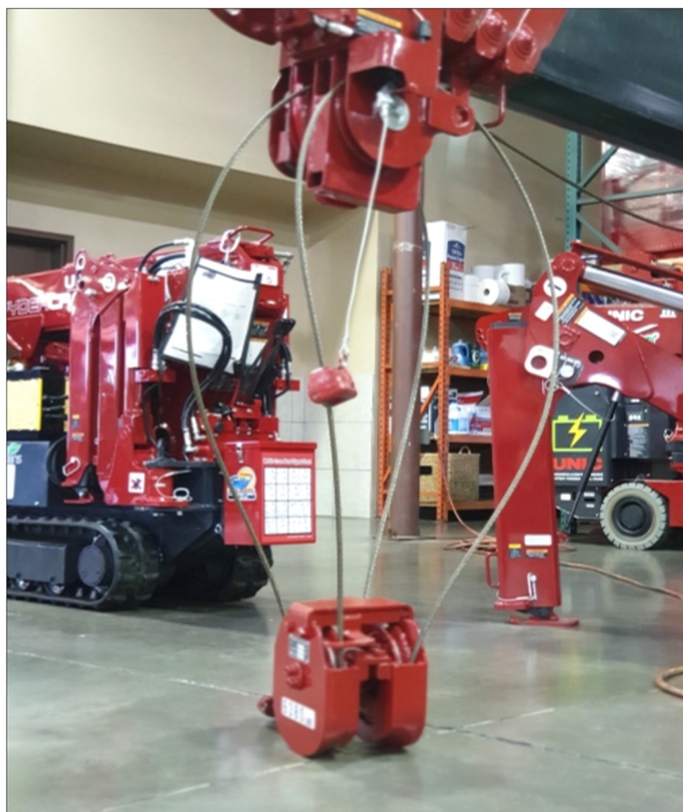
(Fig. 1): NEVER lift the hook block off the ground via WINCHING UP; ALWAYS BOOM UP/BOOM OUT to un-ground the hook block.
