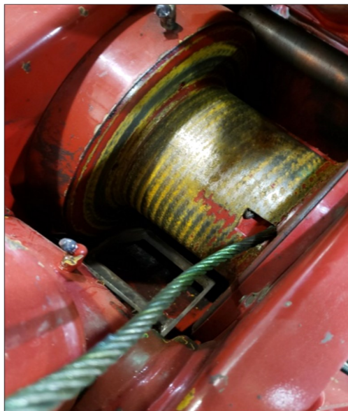
(Fig. 1): Rotate the Wire Rope Drum, until the narrow end of the Wire Rope Wedge is visible.
