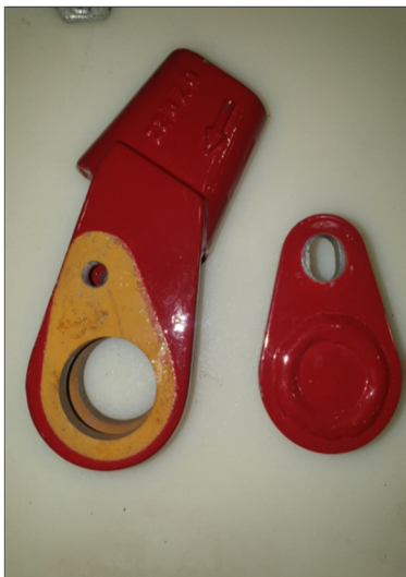
(Fig. 2): The Wire Rope Socket for the 2-Part Hook Block is the same as the 1-Part Hook Block, only uninstalled from the hook body
