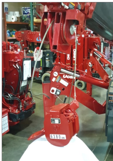
(Fig. 3): Pull the uninstalled wire rope through all of the sheaves of the 4-Part Hook Block and the left-hand sheave of the Boom Tip.
