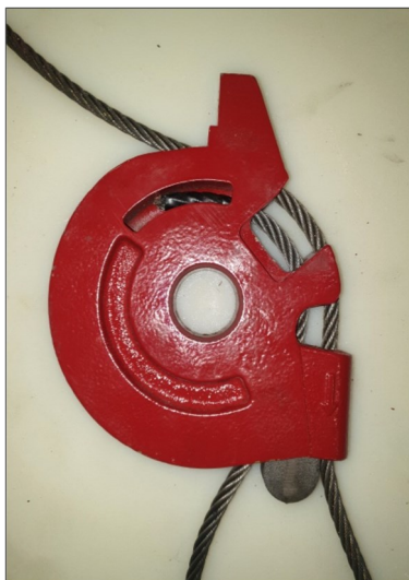
(Fig. 2): Remove (or at least loosen) the Wire Rope Clip before attempting to uninstall the wire rope from the Wire Rope Socket.
