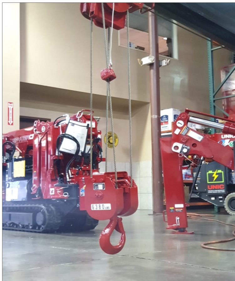
(Fig. 1): WINCH DOWN to lower the hook to the ground, but DO NOT ground the hook via WINCH DOWN.
