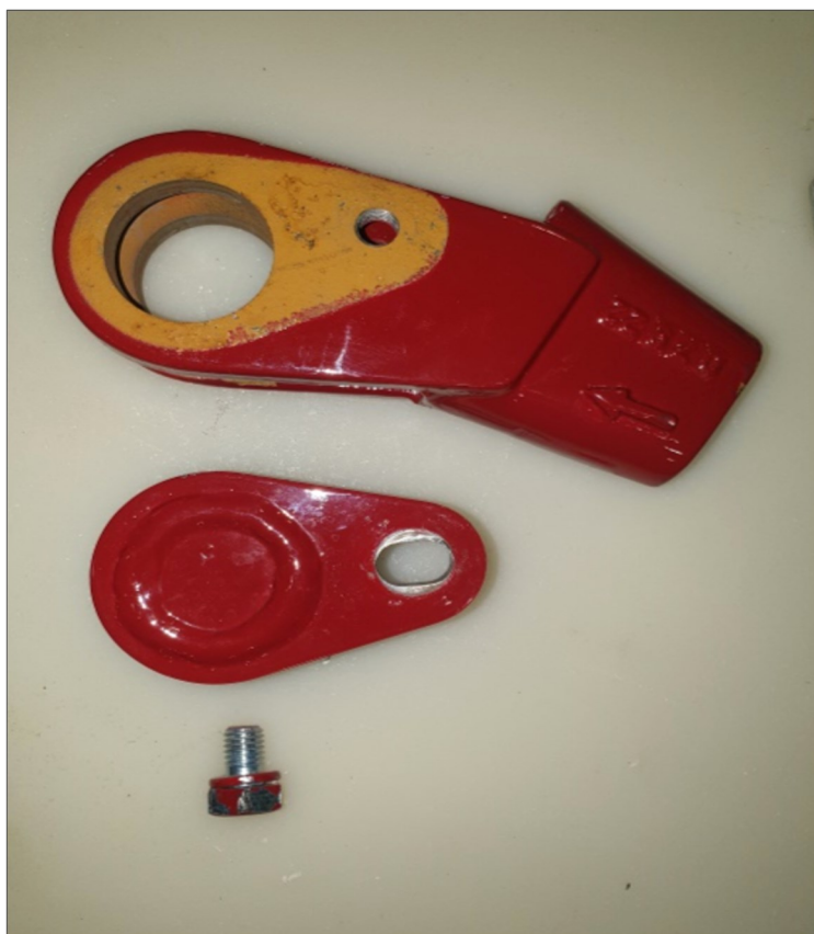
(Fig. 4): The Wire Rope Socket is used with both the 1-Part and 2-Part Hook Blocks
