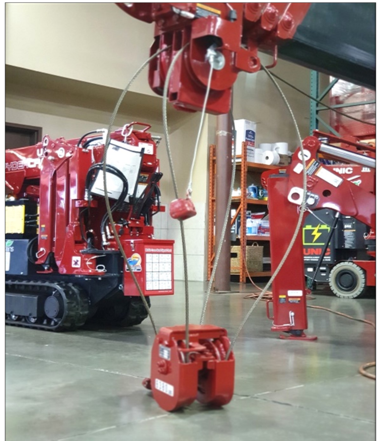
(Fig. 2): BOOM DOWN to actually place the hook block on the ground.
