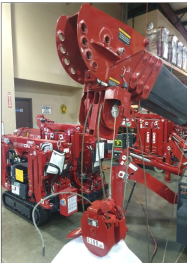
(Fig. 2): Orient the 4-Part Hook so that the A2B Ledge of the hook block is directly below the hanging A2B Weight.
