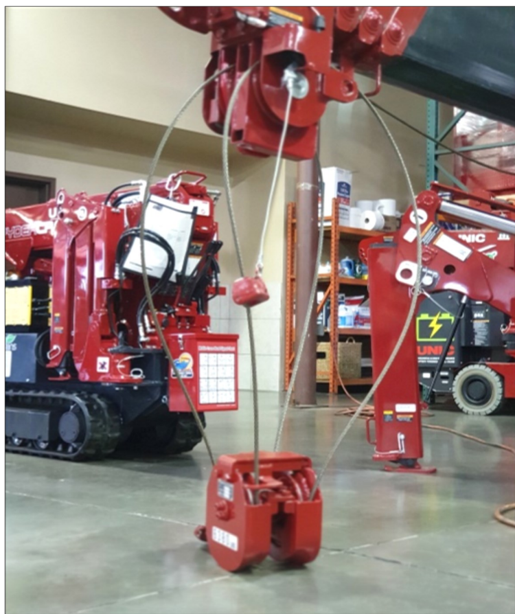
(Fig. 1): NEVER lift the hook block off the ground via WINCHING UP; ALWAYS BOOM UP/BOOM OUT to un-ground the hook block.
