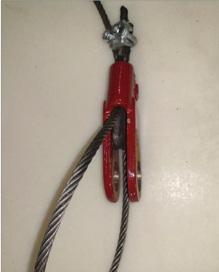
(Fig. 5): Remove the Wire Rope Clip and push out the Wire Rope Wedge from the Wire Rope Socket.
