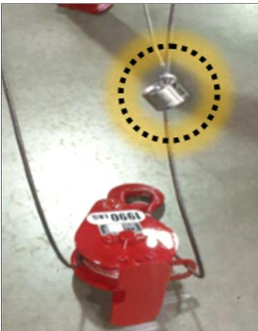
(Fig. 1): The 94- and 95-Series have slightly different 2-Part Hook Block and A2B Weight designs, but the procedure is the same.
