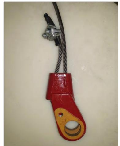
(Fig. 4): Before closing the loop and seating the wedge, ensure there is AT LEAST 6" of "tail" ABOVE the becket.
