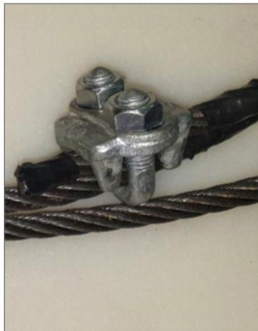
(Fig. 3): When assembling the wire rope clip, make sure to place the U-bolt on the actual wire rope and the saddle on the Wire Rope Spacer.
