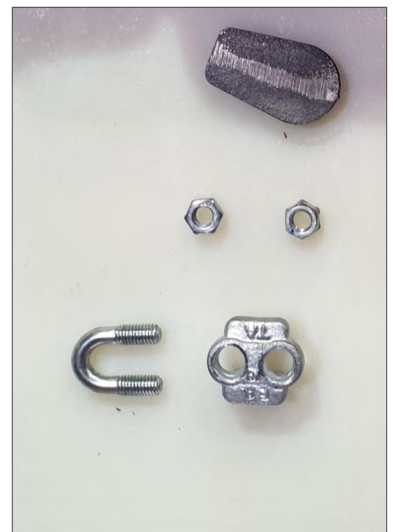
(Fig. 8): Retain the Wire Rope Clip and Wire Rope Socket Wedge after installing the Wire Rope Socket.
