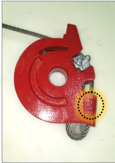
(Fig. 3): When you close the loop, you must ensure that the end of the wire rope is still in the viewing channel.
