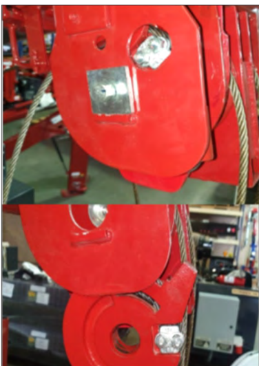
(Fig. 5): Remove the Wire Socket Pin Retention Bolt and then support the Wire Rope Socket as you pull the Wire Rope Socket Pin out.
