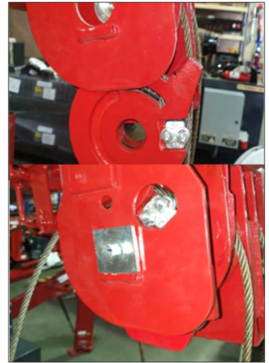
(Fig. 4): When installing the Wire Rope Socket to the Boom Tip, tilt the "tower" of the socket slightly forward and secure with the pin and bolt.
