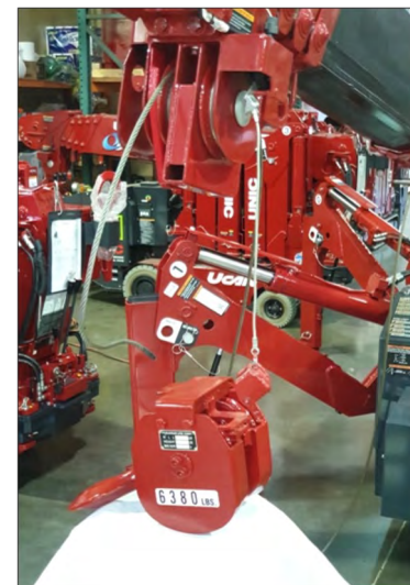
(Fig. 7): Pull the wire rope through all of the sheaves of the 4-Part Hook Block and the left-hand sheave of the Boom Tip.
