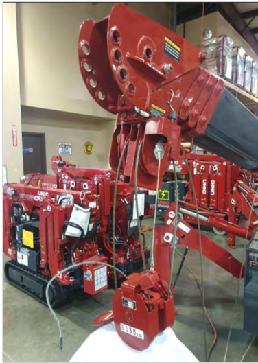
(Fig. 2): Orient the 4-Part Hook Block so that the A2B Weight Ledge of the hook block is directly below the hanging A2B Weight.
