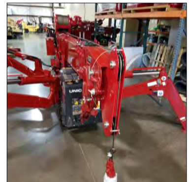
(Fig. 4): The Auxiliary Winch with its wire rope reeved and connected to the 1-Part Hook Block.
