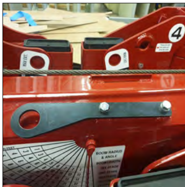
(Fig. 2): The Wire Rope Socket Bracket installed without the Jib Storage Cradle.
