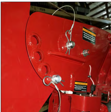
(Fig. 1): The installed Auxiliary Winch BTA with its BTA Pins installed and safety-clipped.
