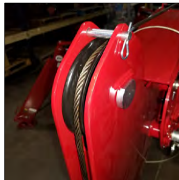
(Fig. 3): The upper Wire Rope Retention Pin, installed.
