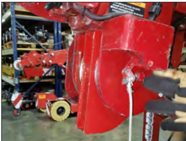
Fig. 1) The Sheave Pin Retaining Bolt and Washer on the left-side of the Boom Tip.
