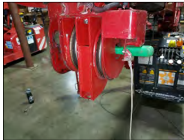
Fig. 2) A prybar used to support the Sheave Assembly with the Sheave Pin removed.
