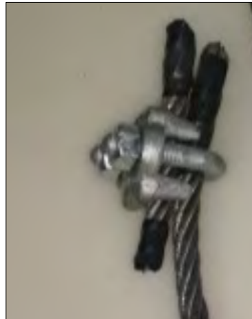
(Fig. 8) The saddle of the Wire Rope Clip sits on the Spacer while the U-Bolt sits on the end of the wire rope.
