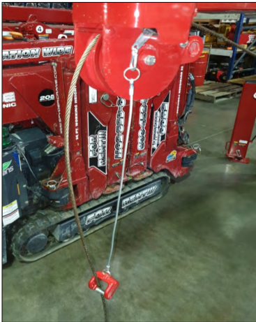
(Fig. 6) The wire rope passes over the right-hand Boom Tip Sheave and Jib Sheave, and through the Jib A2B Weight.
