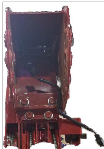
(Fig. 3) The A2B Switch Extension Cord is installed on the inside of the Jib Hood.
