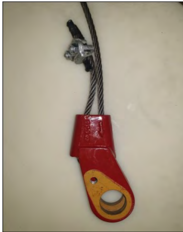
(Fig. 7) Notice the embossed arrow on the side of the becket; the wire rope goes through the narrow end following the arrow.
