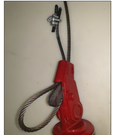
(Fig. 9) Insert the narrow end of the Wire Rope Wedge into the wide side of the becket of the Wire Rope Socket.
