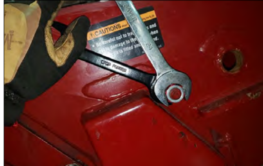
Fig. 5) You will need two 24mm wrenches to remove the Jib Hood Alignment Pin Nuts.
