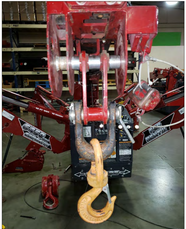
Fig. 6) The Search Hook installed to the boom of the URW295.
