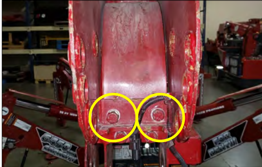
Fig. 4) The 22mm bolts that hold the Jib Hood in-place, indicated by the yellow circles.
