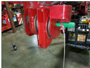
Fig. 2) A prybar used to support the Sheave Assembly with the Sheave Pin removed.
