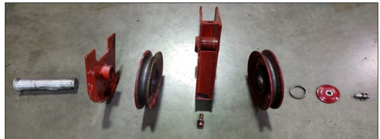
Fig. 3) The Sheave Pin, Wire Rope Guide, right-hand Sheave, Hook Block and Bolt, left-hand Sheave, Spacer, Sheave Pin Retaining Bolt and Washer.
