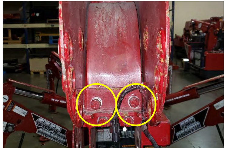
Fig. 5) The 22mm bolts that hold the Jib Hood in-place, indicated by the yellow circles.
