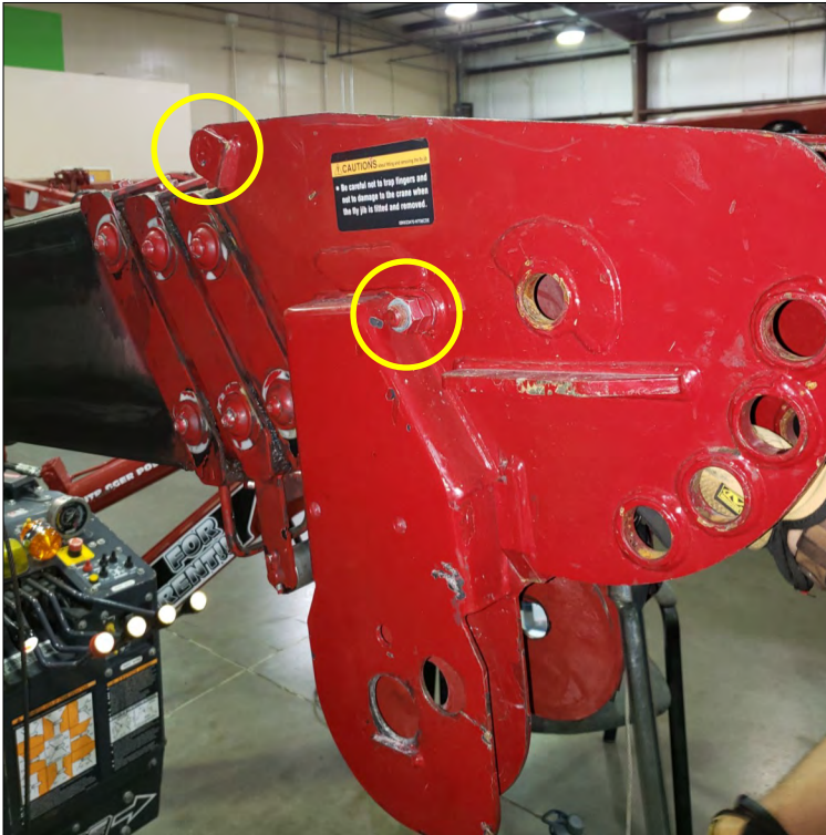
Fig. 3) The Jib Hood Alignment Pin and Jam Nuts and Jib Hood Pin.
