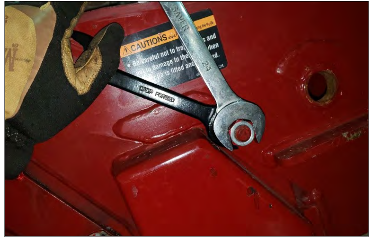
Fig. 5) You will need two 24mm wrenches to install the Jib Hood Alignment Pin Nuts.
