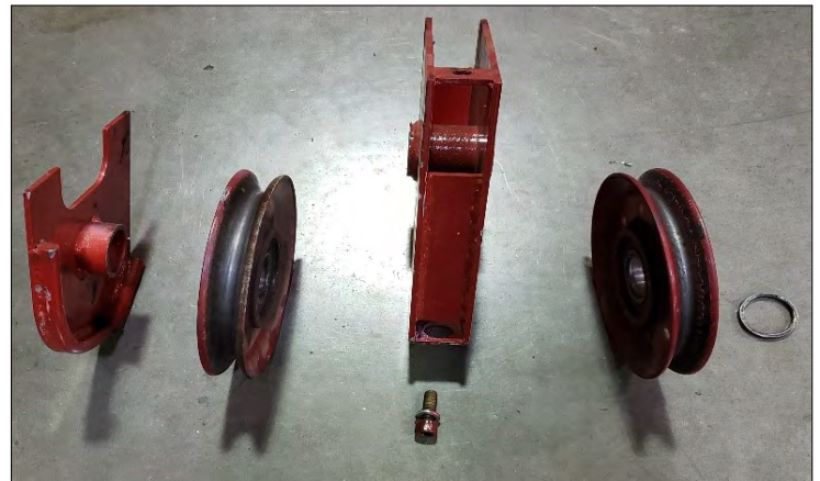
Fig. 1) The Sheave Assembly: the Wire Rope Guide, right-hand Sheave, Hook Block and Bolt, left-hand Sheave, and Spacer.
