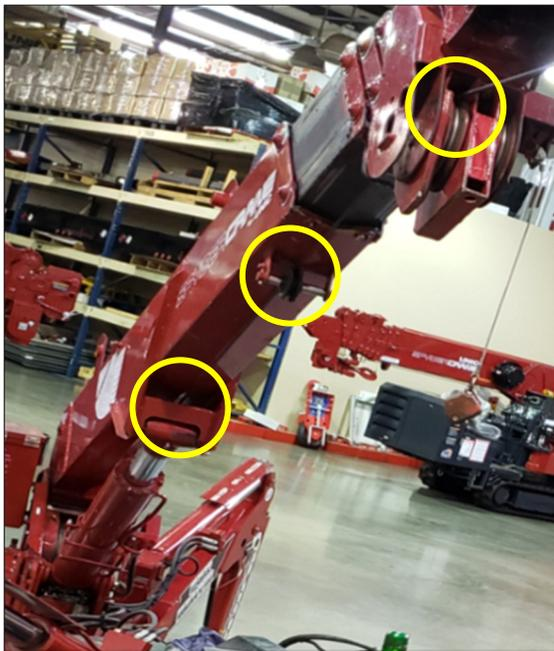
(Fig. 4): Reeve the wire rope through the boom BACKWARDS, starting at the right-hand sheave of the Boom Tip.
